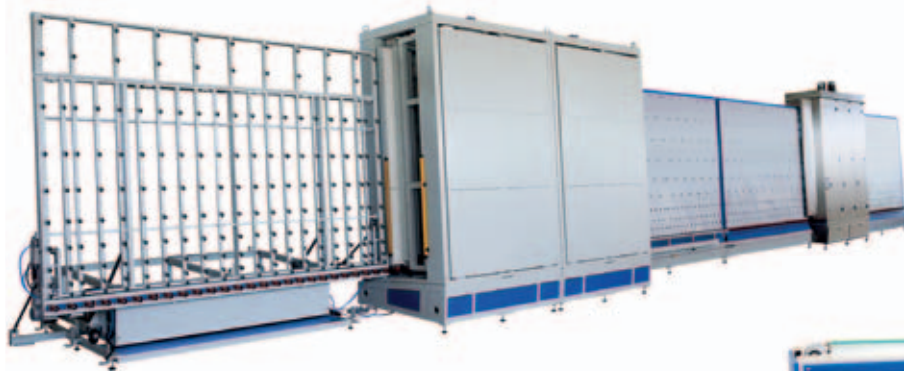
Automatic insulating glass line
