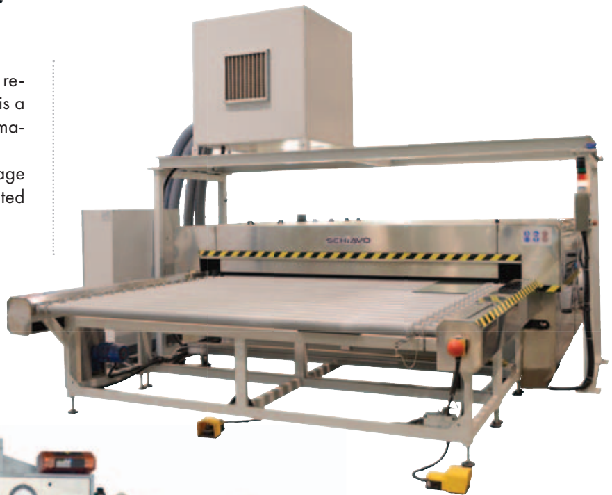
Horizontal glass washing machine HTL2600
