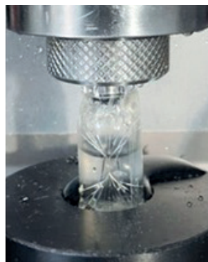
Sample before (left) and after (right) the burst test
