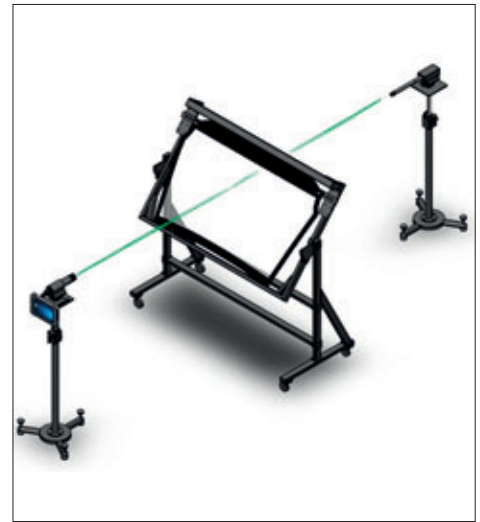
Automatic collimator for ECE R43 secondary image separation
