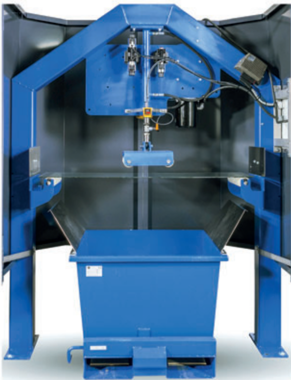
Four point bender for EN1288 mechanical strength testing
