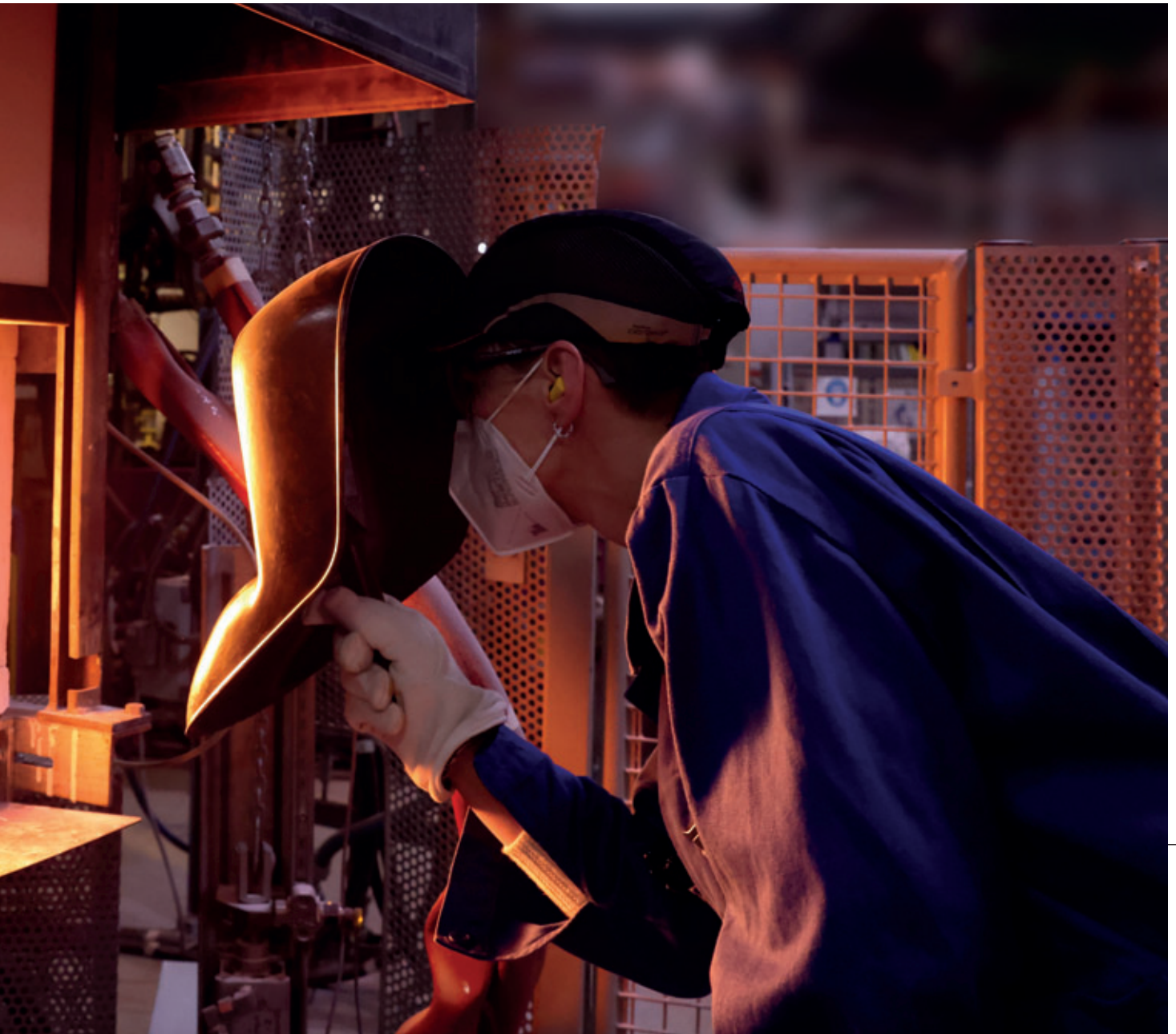
View into the melting tank with liquid glass at up to 1,700 degrees. Photo: courtesy of Schott
