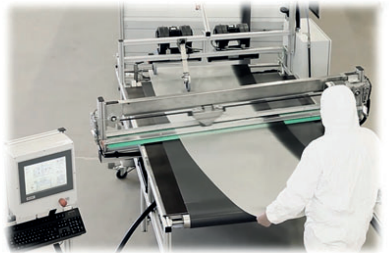
PVB shaping and cutting line
