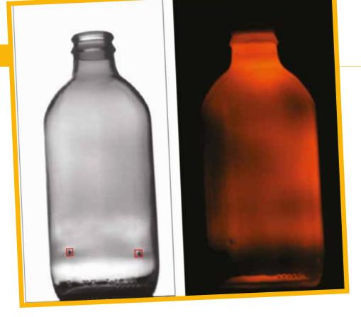
at the hot-end. The high-definition matrix cameras and measurement by transmission both achieve an excellent defect detection level compared to infrared camera technology. Infrared images have areas with different brightness levels creating very dark or very bright areas where it makes it impossible to detect defects. The Tiama HOT eye is not impacted by these differences in radiation - which allows for complete inspection of the article from bottom to finish.
