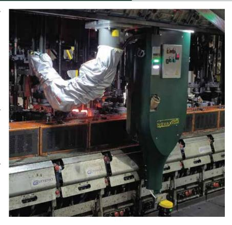
IS machines, this suspended version will provide uncompromising rigidity, which is crucial for maintaining precision during high-speed swabbing processes. Available for both new installations and conversions of existing setups, the NX-SR-300 exemplifies Novaxion's singular efforts to provide adaptable solutions that can cater to the diverse needs of glass manufacturers.
