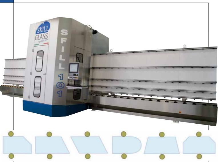
These vertical drilling and milling centres can operate at great speed and precision - thanks to the management of all processes by numerical control as well as double tool change support. Milling on this machine is a simple and quick operation. Indeed by using multiple tools it can mill and grind an insert in just a few seconds just like the polishing that can be carried out in small inserts, with 50 or 30 mm grinders.
