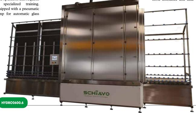
exchange capabilities. The HYDRO model handles glass heights from 1600 to 3300 mm and thicknesses up to 40 mm.
