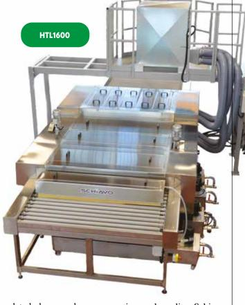
sulated glass panels, capable of handling dimensions up to 6000x3300 mm.
