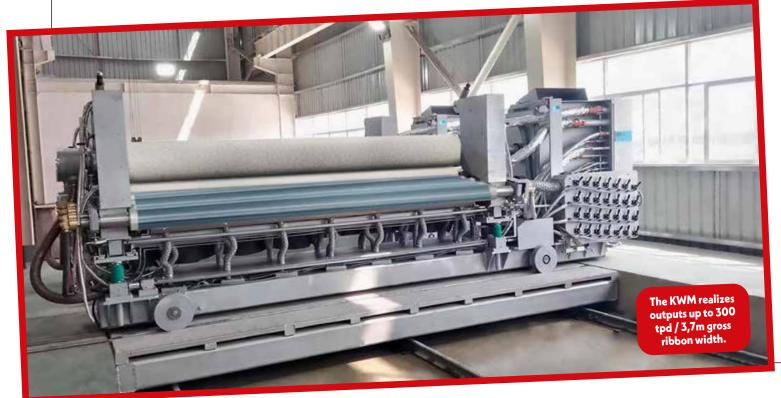
the desired thickness and further processed. The KWM 8s Line boasts an impressive capacity, effortlessly handling up to 300 tons of glass per day. This remarkable output is complemented by its versatility, seamlessly producing flat glass for a wide spectrum of applications, from solar modules to countless other architectural and industrial uses.
